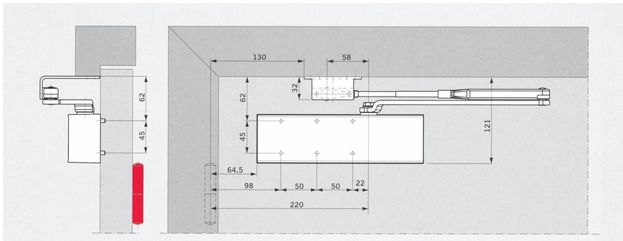
With this fixing method, the max closing force is approx. 20 Nm (for doors up to 950mm)
