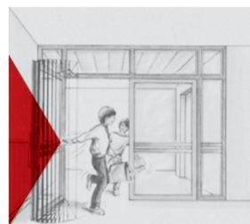
If the DORMA TS 72 is installed with a **hold-open arm**, the doors can be held open at any desired point (up to approx. 150°).
